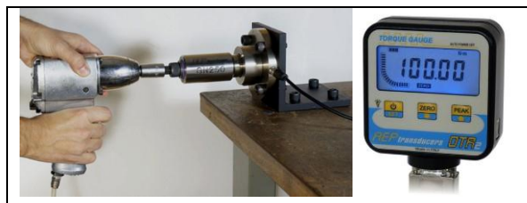
DTR2 + TRF STATIC Torsiometer. System for calibrating impact wrenches
